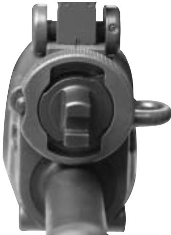
*Position II* (Rib of gas valve in slanting position)
