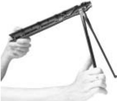
*Remove bipod carrier from the handguard*
