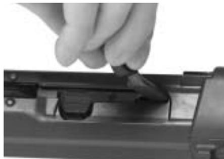
Push bolt to the rear, using bolt handle
