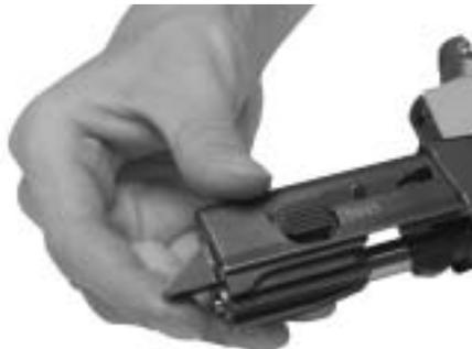
*Inserting the bolt assembly*
